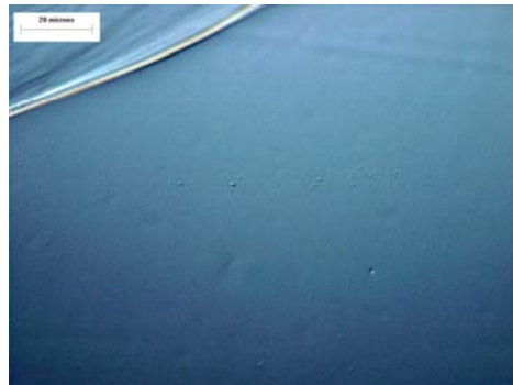
Figure 8b. Optical micrograph of a smooth PhotoLink coating on a device. Note the coating defect in the upper left-hand corner.
