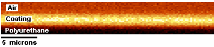
Figure 4. Raman cross-sectional image of coating on polyurethane catheter.
