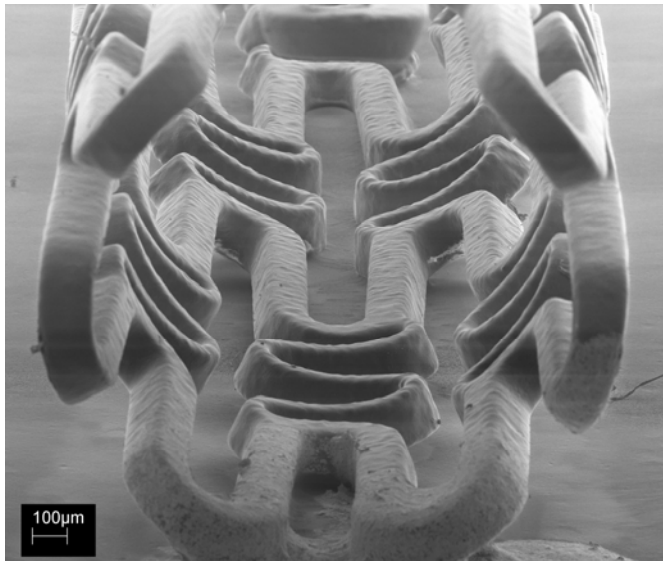
Figure 9. Scanning electron micrograph (SEM) of a drug elution coated stent.
